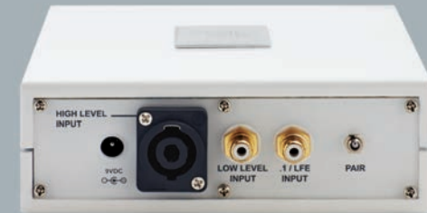
Below: Rear panel of Longbow Wireless Transmitter featuring High Level, .1/LFE and Low Level inputs. High Level and .1/LFE can be run concurrently to permit REL Reference Theater operation that re-establishes consistent, full range bass in addition to special effects bass
